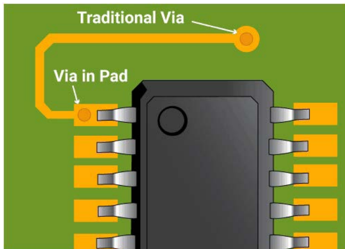
Via-In-Pad Vs. Traditional Via
