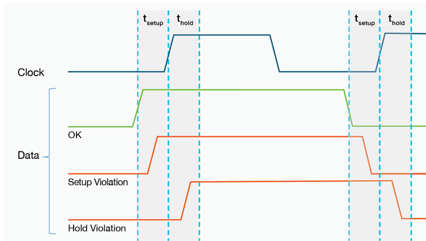
Figure 3.4: Setup and hold time violation signal diagram. Source: https://www.designnews.com/electronics-test/how-track-down-setup-and-hold-violations-mixed-signal-oscilloscope
