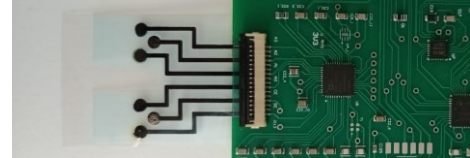
Fig. 4. Proposed flexible sweat sensor connected to the implemented multi-sense PCB via the FD9 connector.
