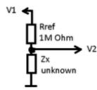
According to Ohm's law, the ratio of voltages V1 and V2 in the circuit is:
