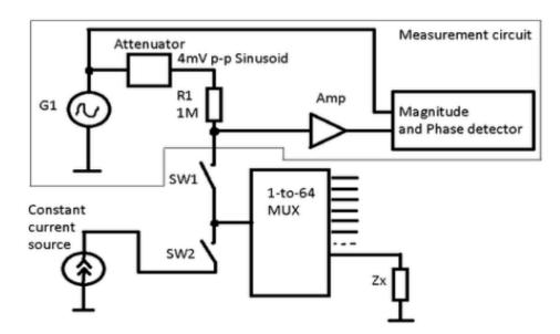
Either the impedance measurement circuit or the electroplating constant current source can be connected to a channel via switches SW1 and SW2.
