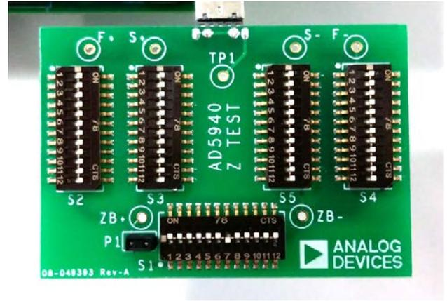
Figure 16. AD5940 Z Test Board Configuration
